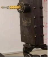
Upconverter and Downconverter assemblies at 38 and 60 GHz, newer ones built at 28 GHz, 72 GHz
