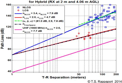
$PL_0$  is path loss measured at close-in distance  $d_0$
