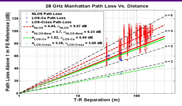
Each point on scatter plot represents a unique pointing angle for TX and RX horn antennas
