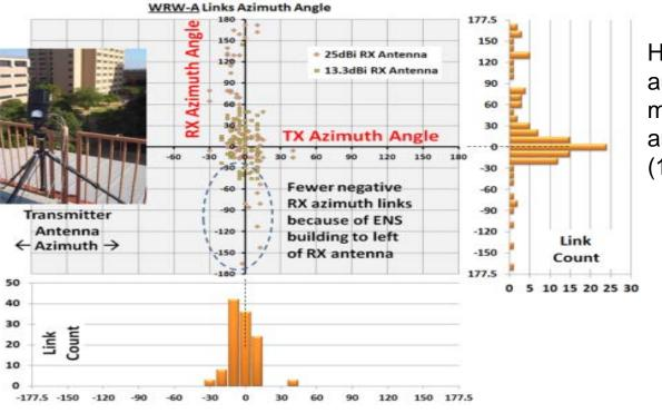
Histogram of RX angles for all links made using 25dBi antennas (10° bins)
