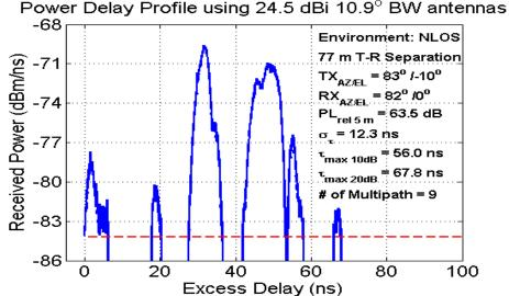
Signals were received at 23 out of 36 RX azimuth angles (10 degree increments)
