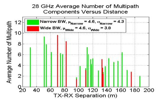
Average number of multipath components (MPCs) per distance: First increases and then decreases with the increasing distance
